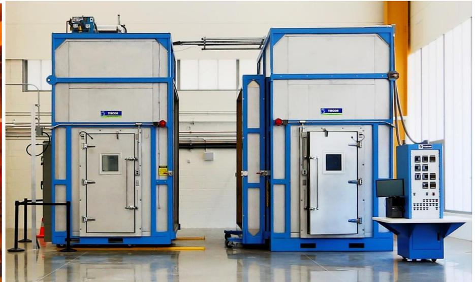
ASTM E283/E2357 Air Leakage Test Apparatus at ORNL
