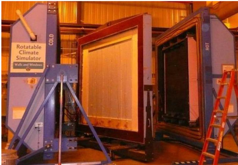
ASTM C1363 Hot Box Test Apparatus at ORNL
