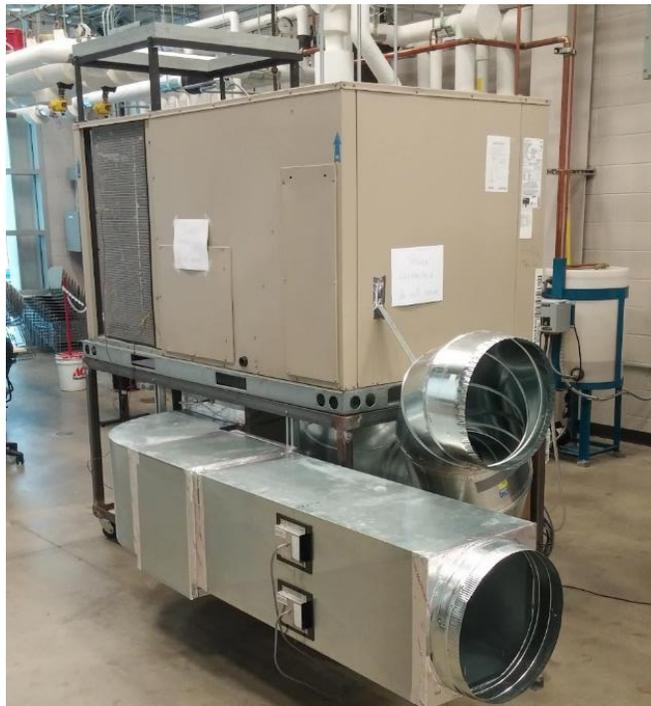
Figure 2.3. RTU used to test automated VRC sensor training kit and evaluate performance of VRC sensor applied to RTU with different types of expansion valves and condenser coils.
