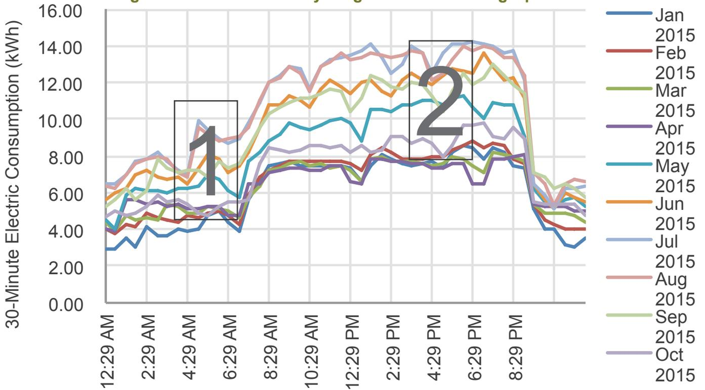
1. Area 1 energy profile curves spike. This fluctuation suggests that there is improperly programmed HVAC equipment or that refrigeration equipment is cycling instead of coasting
