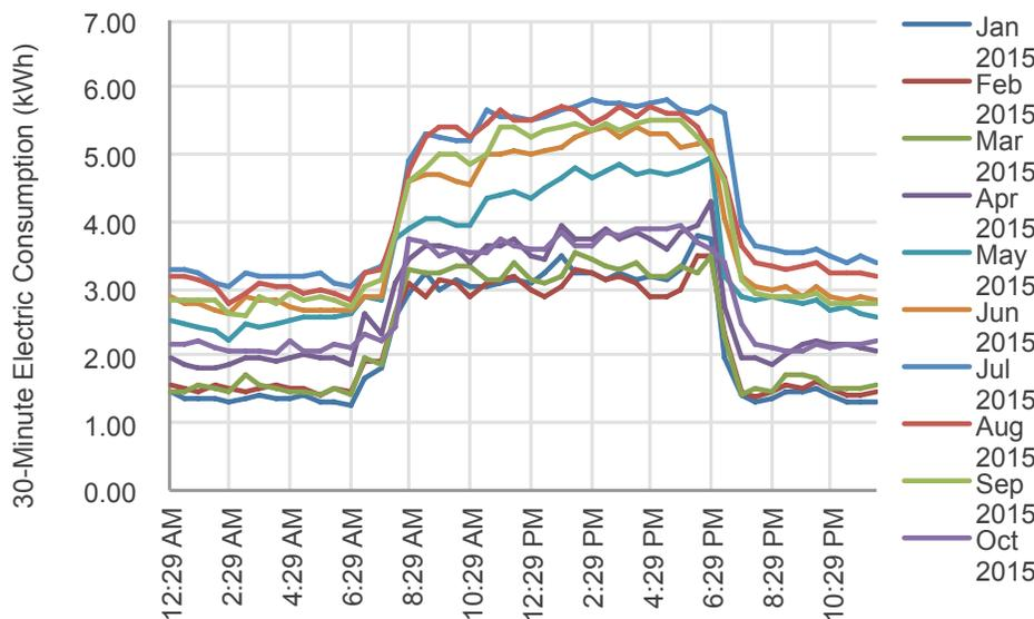
Store 1 shows normal interval data curves, where energy use consistently increases during operating hours. This data shows how summer month electric energy consumption is higher than peak and winter months. Store 1 has case heat service.
