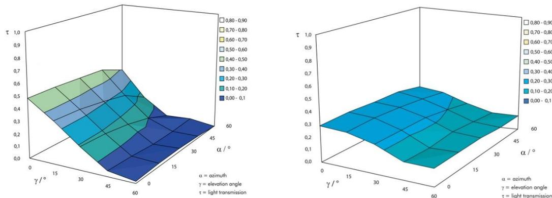
Figure 25 Daylight-optimized louver geometries ensure solar heat control based on the sun’s angle of incidence (Koester, 2012)
