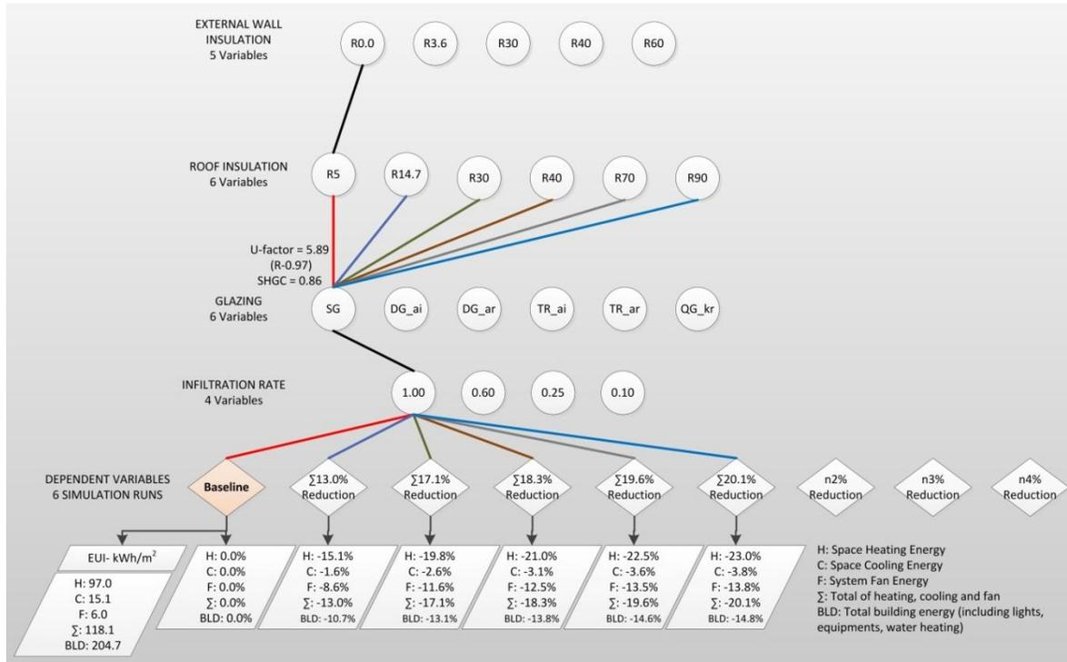
Figure 13 Parametric tree for roof thermal insulation alternatives (Karaguzel & Lam, 2012)
