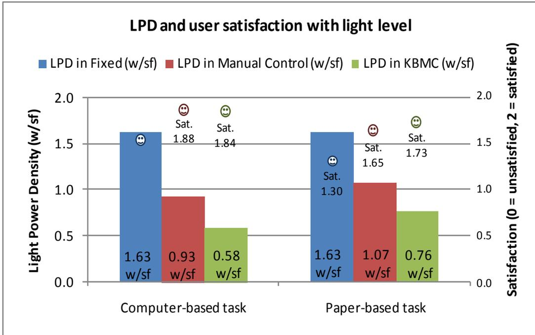
Figure 26 Manual Control of blinds, task and overhead lighting provide energy savings over fixed ceiling based task ambient lighting (Gu, 2011)
