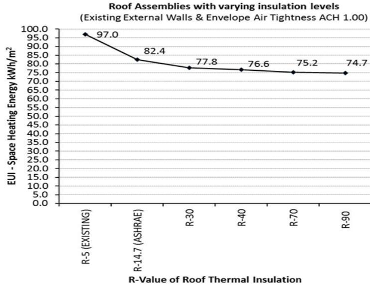
Figure 12 Effects of roof thermal insulation thickness on space heating energy consumption (Karaguzel & Lam, 2012)
