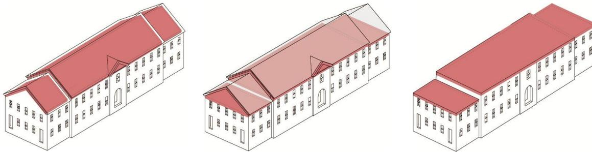
Figure 15 Three common roof insulation variations in retrofit applications
