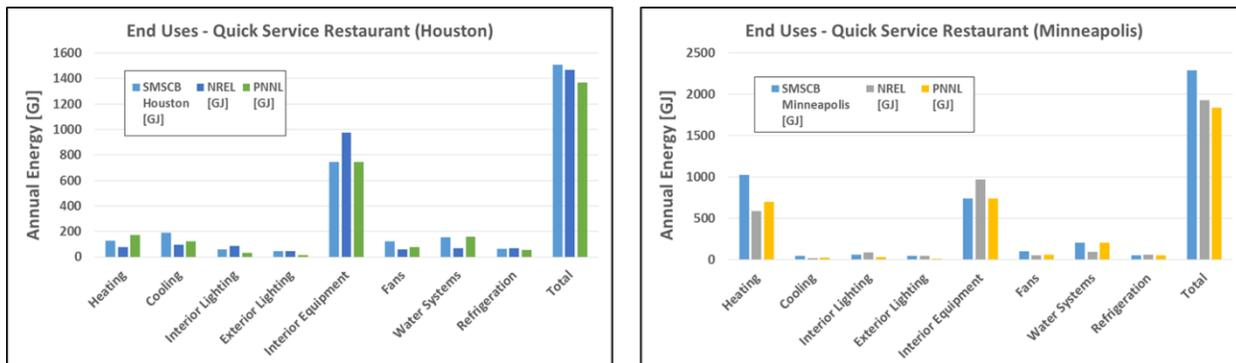
Figure 1. Annual Energy Consumption Comparison with PNNL and NREL Reference Models for Quick Service Restaurant
