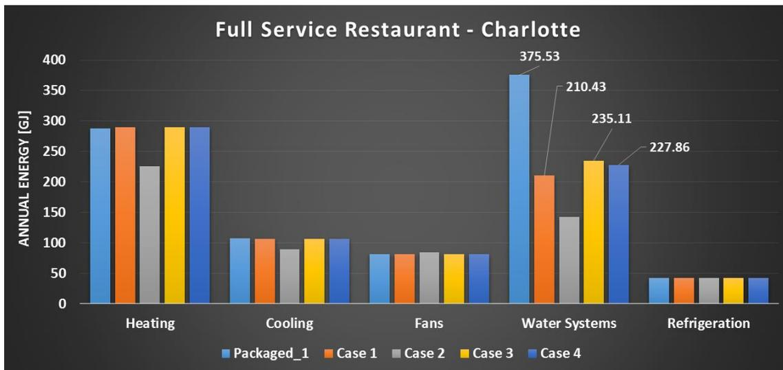
Figure 13. Energy Comparison of Retrofit Water System for Full Service Restaurant in Charlotte
