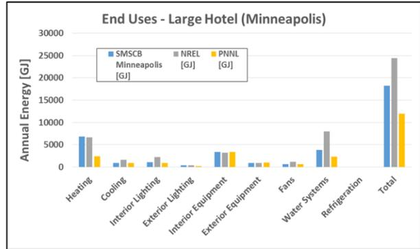
Figure 4. Annual Energy Consumption Comparison with PNNL and NREL Reference Models for Large Hotel
