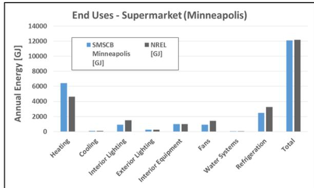
Figure 5. Annual Energy Consumption Comparison with PNNL and NREL Reference Models for Supermarket
