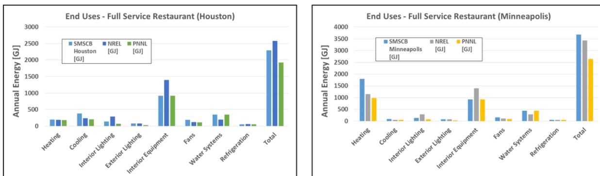
Figure 2. Annual Energy Consumption Comparison with PNNL and NREL Reference Models for Full Service Restaurant
