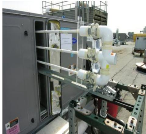
Figure 3.12 Air sampling tree on AC24F
