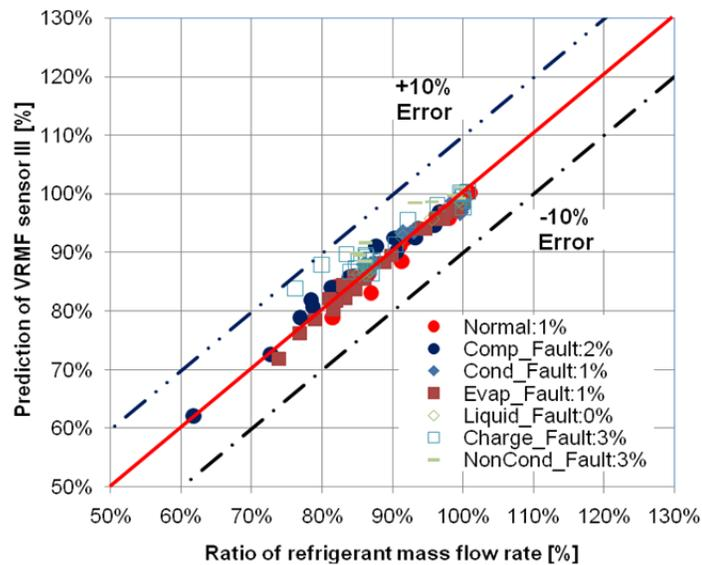
Figure 3.33 Performance of VRMF sensors III based on TXV model under no fault and fault conditions
