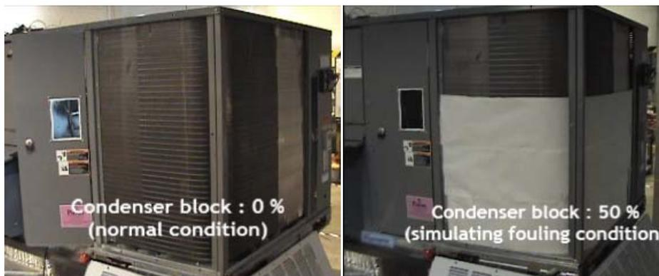
Figure 3.88 Condenser status of RTU system (left side: normal & right side: 50% blocking)
