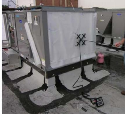
Figure 3.15 Measurements of speed of air entering the first-circuit condenser
