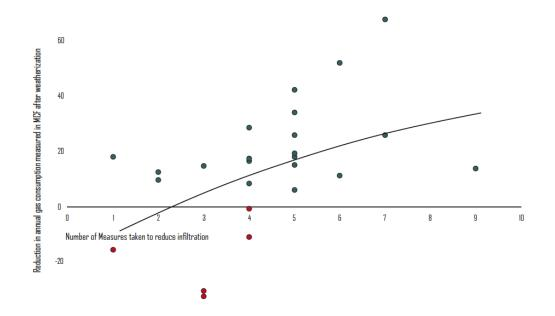
Figure 11 Effect of measures taken to reduce infiltration on annual gas consumption (Tanski, Loftness, Aziz, & Cochran, 2011)
