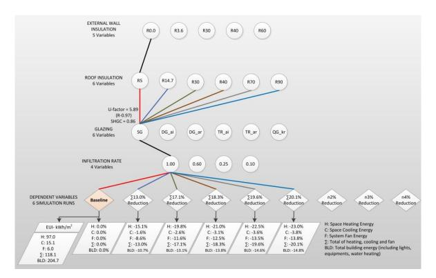
*Figure 13 Parametric tree for roof thermal insulation alternatives (Karaguzel & Lam, 2012)*
