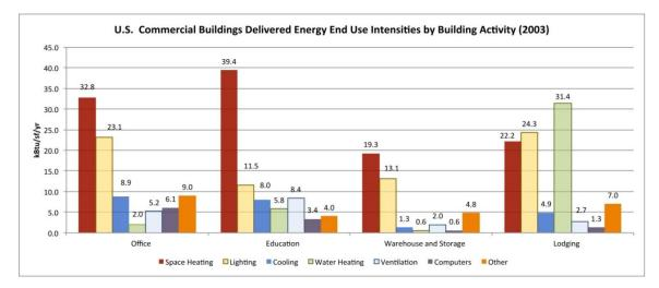
Figure 1 Heating and lighting are the dominant energy loads in four building types (CBECS 2003)
