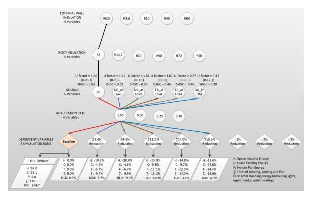
Figure 14 Parametric tree for glazing alternatives (Karaguzel & Lam, 2012)
