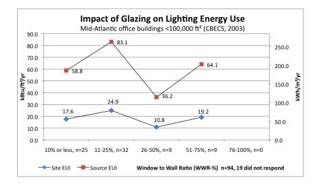
Figure 28 Window area and specification has a significant impact on lighting energy (CBECS , 2003)
