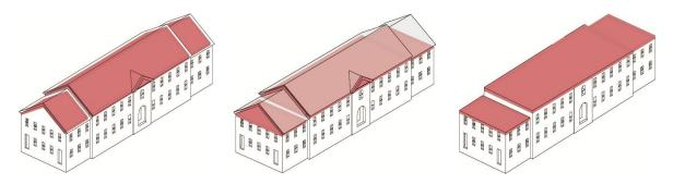
Figure 15 Three common roof insulation variations in retrofit applications
