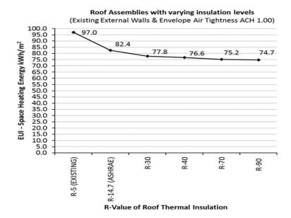
Figure 12 Effects of roof thermal insulation thickness on space heating energy consumption (Karaguzel & Lam, 2012)
