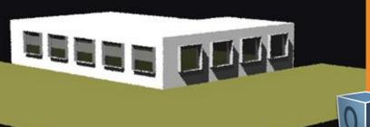
New Radiance daylight calculation programs are utilized by an OpenStudio measure to enhance OpenStudio's daylight modeling. These enhancements expand the complexity of daylight modeling and enhance the analysis of lighting energy savings in daylight area control zones. Additional features include the calculation of space-by-space and fullbuilding Spatial Daylight Autonomy (SDA) and Annual Sunlight Exposure (ASE) analysis, as specified in the most recent version of LEED (LEED v4).
