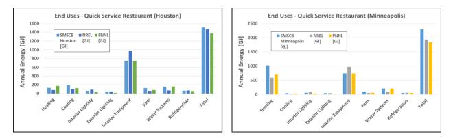
Figure 1. Annual Energy Consumption Comparison with PNNL and NREL Reference Models for Quick Service Restaurant
