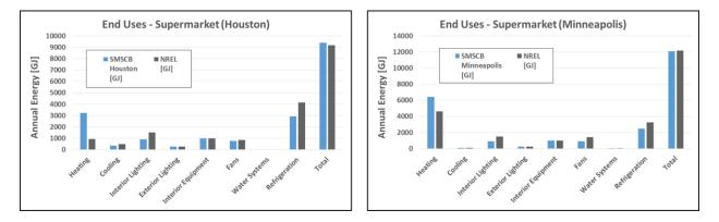
Figure 5. Annual Energy Consumption Comparison with PNNL and NREL Reference Models for Supermarket
