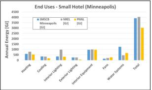
Figure 3. Annual Energy Consumption Comparison with PNNL and NREL Reference Models for Small Hotel
