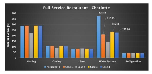
Figure 13. Energy Comparison of Retrofit Water System for Full Service Restaurant in Charlotte
